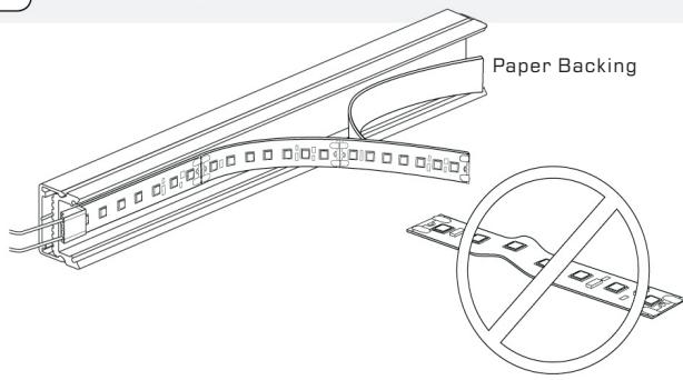
Attach the quick connector or solder lead wires to one side of the tape. Shorten the LED tape to desired length by cutting along the marked area in between the solder pads. Remove paper backing from the adhesive tape firmly press down onto the aluminum surface. Uncoil and peel minimal amount as you install to avoid collection of debris. Excessive uncoiling and peeling of tape create ripples and air bubbles on the tape that should be avoided.
