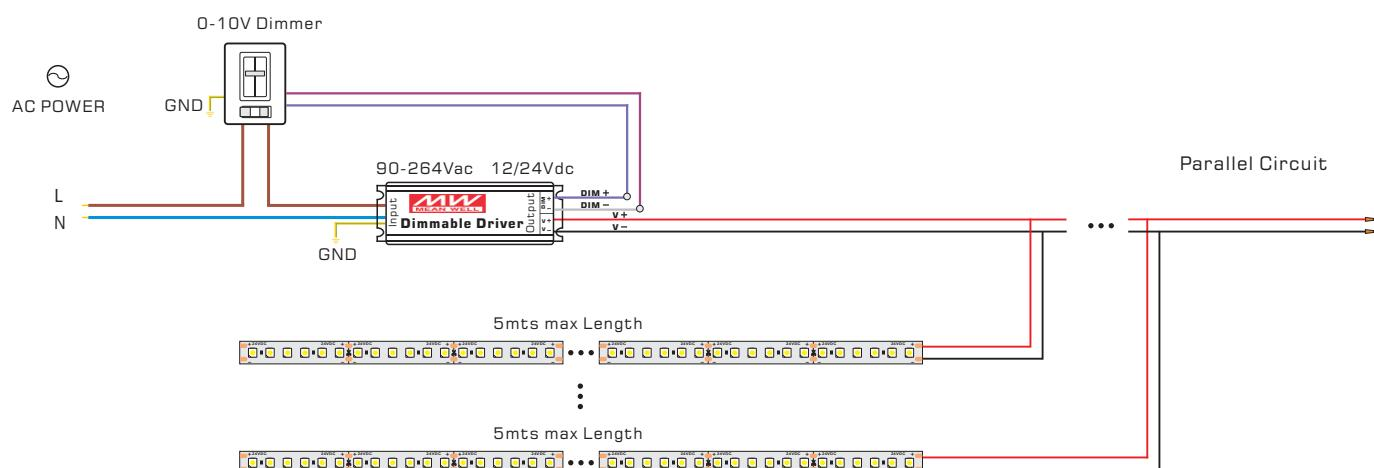
\* Wire section suitable to length and load of installation
