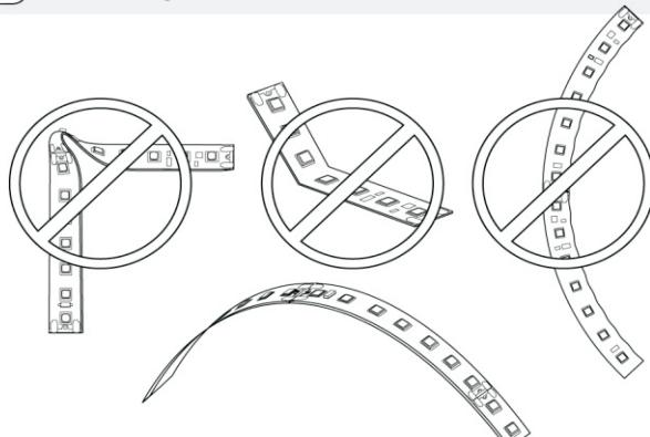
Mechanical stress of the tape must absolutely be avoided. Assembly must not lead to damage or interruption of the circuit paths. Avoid Electro-static Discharge with proper equipment. Do not attempt to bend the tape horizontally or with sharp edges.
