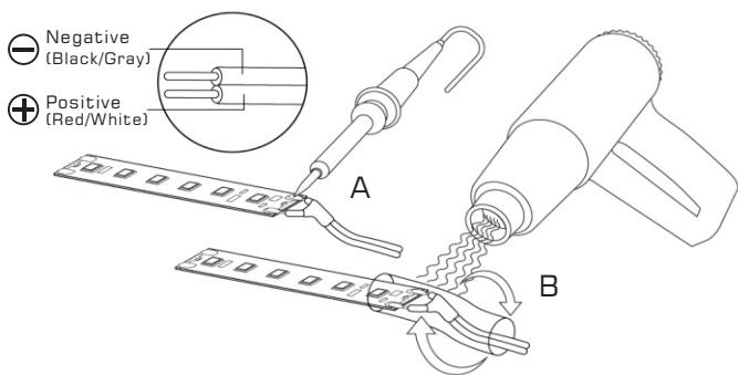
Lead wires can be soldered onto the tape. Solder connections should only be performed manually on designated solder pads that are marked as "24 V"(A). The maximum solder time is 3 seconds and the maximum soldering temperature is 662°F (350°C). After soldering, use shrink tube (provided by others) over the connection and cure with heat gun (B).
