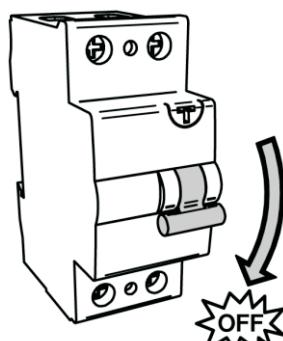
Turn off all the power before installing the LED strips & Aluminum profiles
