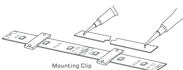
For additional security, use mounting clips every 12" (supplied by others) or apply small amounts of epoxy at each end to increase holding force. Refer to table for recommended epoxy brands. Avoid installing the tape overhead without taking additional securing measures.
