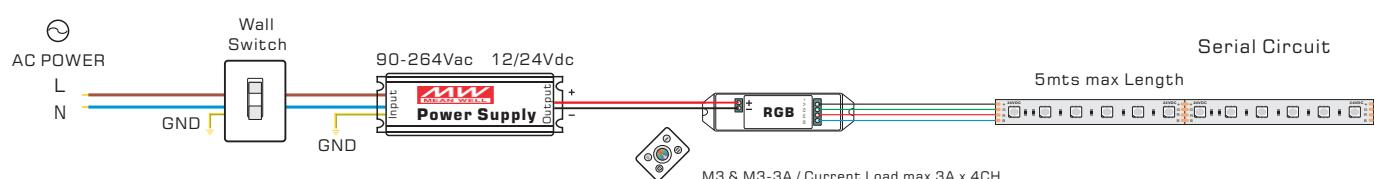
\* Wire section suitable to length and load of installation
