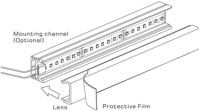
Snap the diffuser lens into the aluminum extrusion. Remove the protective film from the diffuser lens.
