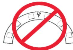
**DO NOT** bend LED strips light to a diameter less than **6cm**.
