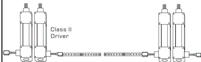
Maximum run length of the tape depends on the power supply specifications. For continuous runs, place the power supplies either at both ends of the run or in the middle of the run next to each other.
