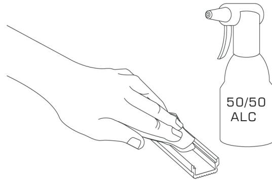
Thoroughly clean the area where tape lights will be installed. Using a 50/50 alcohol mix, clean the area where LEDs will be applied and allow time for alcohol to dry for 5 minutes.
