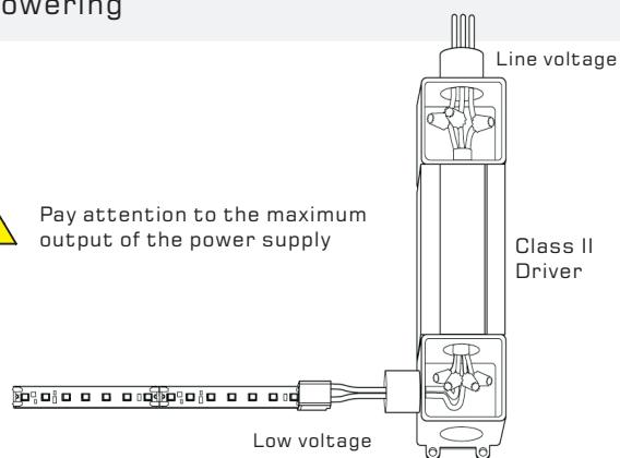
Connect positive wire to RED (white) low voltage wire from power supply. Also, connect negative wires to BLACK (gray) low voltage wire from power supply. Refer to the power supply data sheets for the maximum cable length from power supply to the product.
