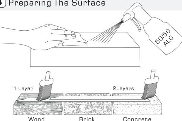
Wipe the surface with 50/50 alcohol solution to provide a clean mounting surface, free of oils, silicones and dirt particles. The mounting surface must have be smooth and have sufficient structural integrity. For porous materials like wood, brick or concrete, optional painting / priming the surface increases bonding power.
