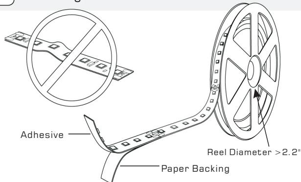
The tape shall only be mounted on surfaces that provide sufficient cooling. Remove the paper backing from the tape and firmly press down onto the surface. Uncoil and peel the minimal amount of tape as you install to avoid collection of debris. Excessive uncoiling and peeling create ripples and air bubbles on the tape that should be avoided.
