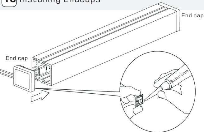
Feed the lead wires through or behind the endcap. Add Super Glue inside and around end cap to secure it in place. For select models, use torque bit to screw the endcap. If applicable, secure the Quick Connector by adding super glue and pressing it onto the extrusion.
