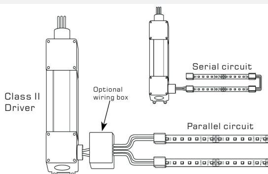
Parallel drive circuits ensure a safer operation (A). Use an optional wiring box to split parallel circuits. Refer to product data sheet for further information. If used with serial circuit (B), the maximum length of a single unit to be driven in series equals the maximum length of the tape. If exceeded, asymmetric voltage drops can lead to a strong over current and damage of single modules.
