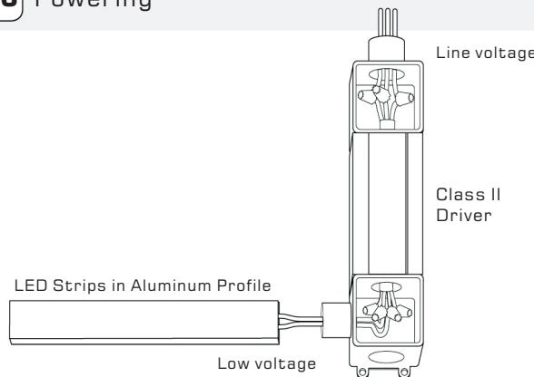
Ensure the correct (wattage & voltage) power supply is used to power the tape. Then proceed to connect low voltage wires from extrusion to power supply. For more information please refer to power supply and LED tape wiring instructions.
