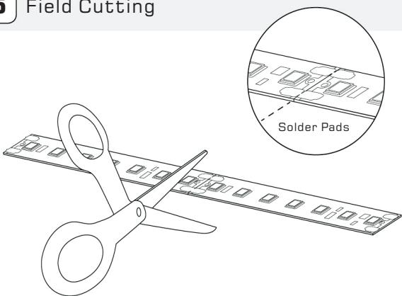
The tape can be cut with a pair of scissors at marked locations in between solder pads. Refer to the product datasheet for exact cut lengths. Always cut from end with no connector/wire leads. Then use either soldering or Quick Connect methods to power cut sections.
